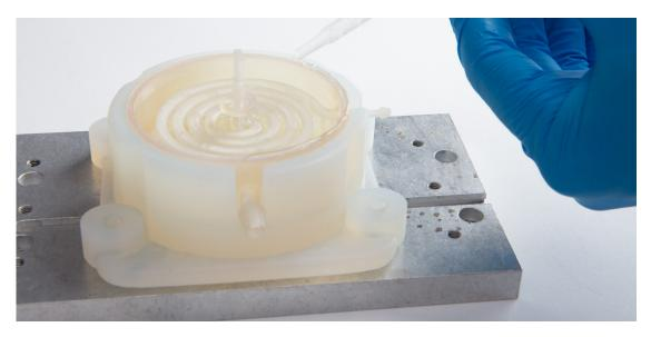
Adhesive being applied to a part in a bonding jig printed in Formlabs Durable Resin.
