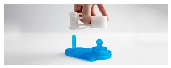
A locating jig designed for minimal contact, printed in Formlabs Tough Resin.
