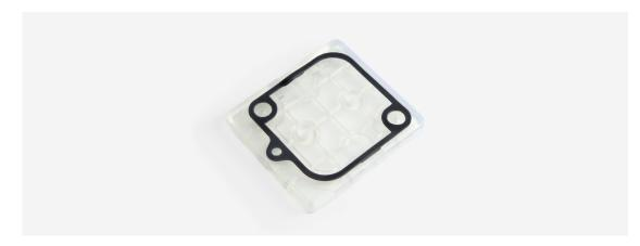
A go/no go gauge for inspecting a rubber gasket, printed in Formlabs Clear Resin.
