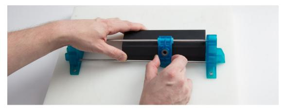
The drill jig slides smoothly across the steel rails by using Formlabs Durable Resin bushings pressed into the Tough Resin guide.
