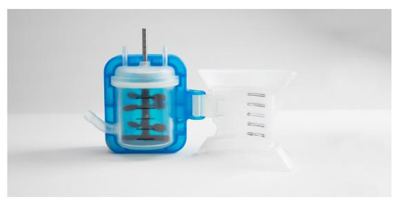
Hinged jig for applying volumetric markings, printed with Formlabs Tough Resin and Durable Resin.
