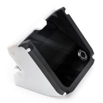
An assembly jig used for manufacturing the Formlabs Form 2 3D printer.
