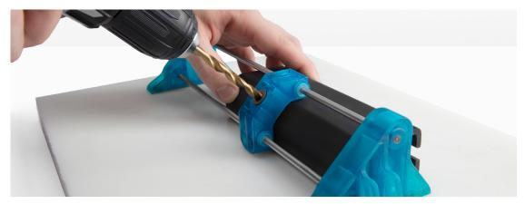
A press fit bushing in a drill jig, printed in Formlabs Tough Resin.
