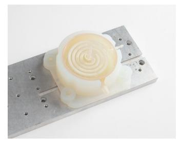
A part properly seated in a pocket jig printed in Formlabs Durable Resin.
