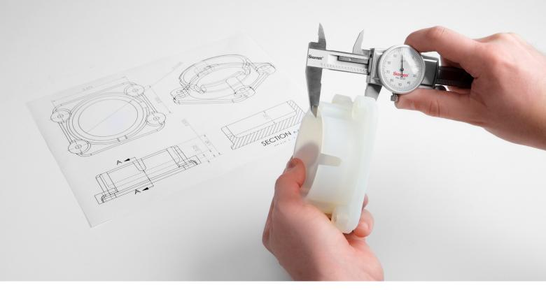
Inspecting a 3D printed part with a caliper to verify dimensional accuracy.
