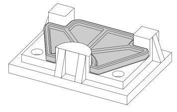
A typical milled geometry for minimizing material removal and machining time.
