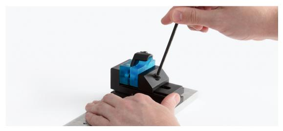
A part being clamped between soft jaw inserts, printed in Formlabs Tough Resin.
