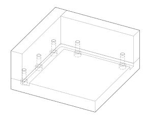
A typical milled and assembled corner locator, composed of three bolted plates, creates more opportunities for chips to become wedged.
