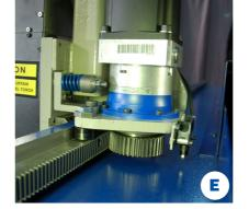
Y-AXIS DRIVE Linear ways combined with Messer's SureTrack pitch line gear engagement to ensure long life and precise motion.
