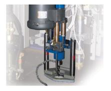
ELECTRIC DRILL UNIT Maximum drill diameter is 1/2". Combined with plasma and oxy-fuel cutting allows for more work to be done on the piece part in a single handling. (Optional)
