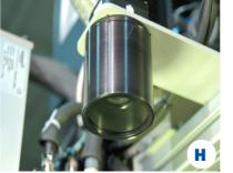
The on-board video camera can be used as an alignment tool and to monitor the cutting process. The image is conveniently displayed on the 24" TFT color screen of the Global Control Plus. (Optional)
