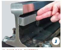
X-AXIS RAIL SYSTEM Over-sized floor mounted rail provides a rigid foundation for smooth, stable machine motion. Fast, accurate installation is assured with Messer's exclusive precision leveling and alignment pads.
