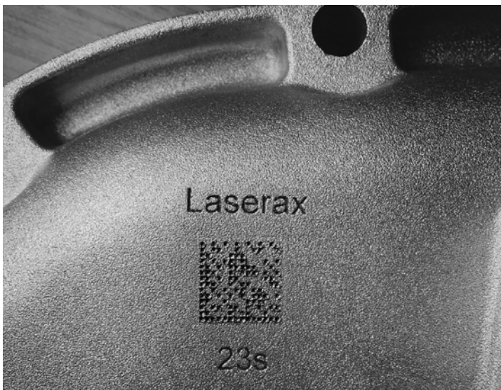
Figure 3 - Photos of a DMC etched using Laserax's shotblast resistant marking a) before shotblast and b) after shotblast
