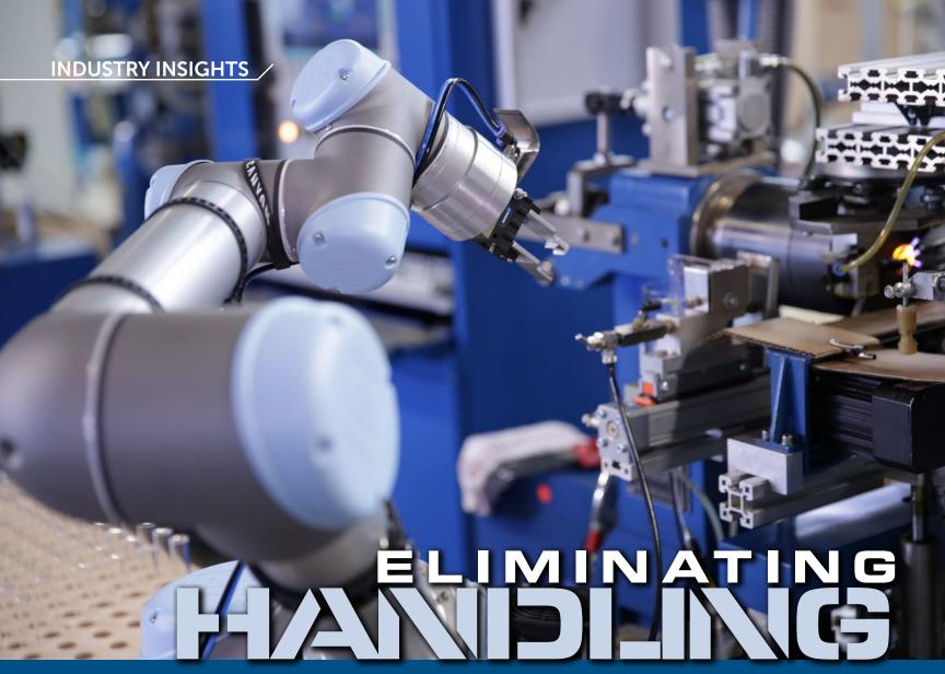
Collaborative robots take over manual handling of glass tubes in CNC glass lathe, increase capacity 50%
